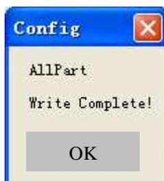
Write operations, you need to pay attention **"to read and write target"** option. Write **ROM** data is not lost after power-down, write **RAM** data will be lost after power-down, but some parameters can take effect immediately (without restarting equipment with immediate effect). Also proposes to select the ROM and RAM in the same time for write operation.
