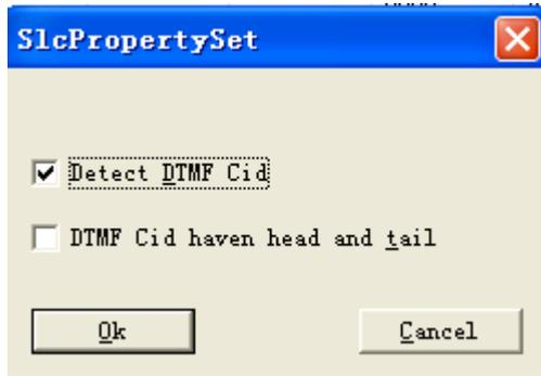
When you need to determine the beginning and end of DTMF call signs, in the "analog line" parameter setting page as below:
